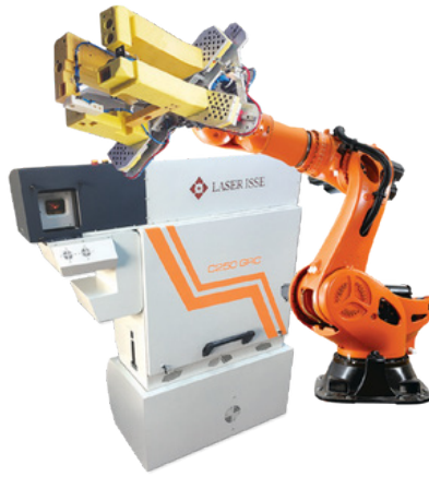
Robotic Laser Marking
